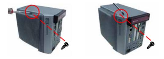
Step 4 Open the top cover and locate the two Hard Disk Drives from the side.
